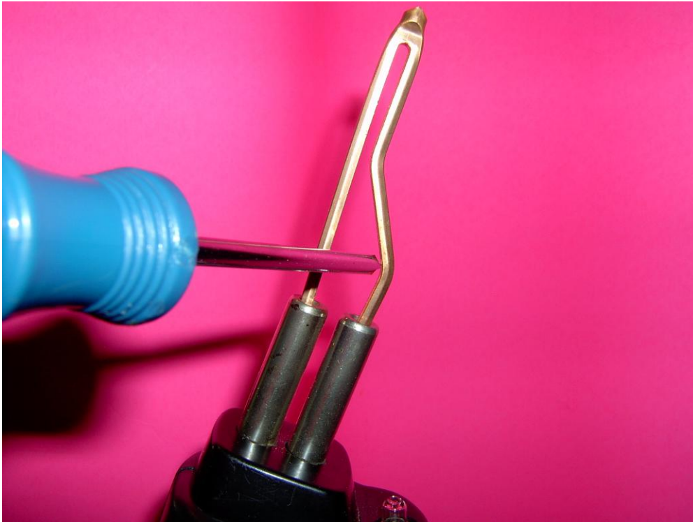
A Philips Head Screwdriver being de-magnetized with a Soldering Gun
