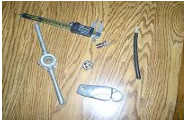
Scrap piece of RG-8 style coax and tools. Precision Calipers, PL-259, Die Holder, 7/16 X 14 Die and a Coax Cutter.
