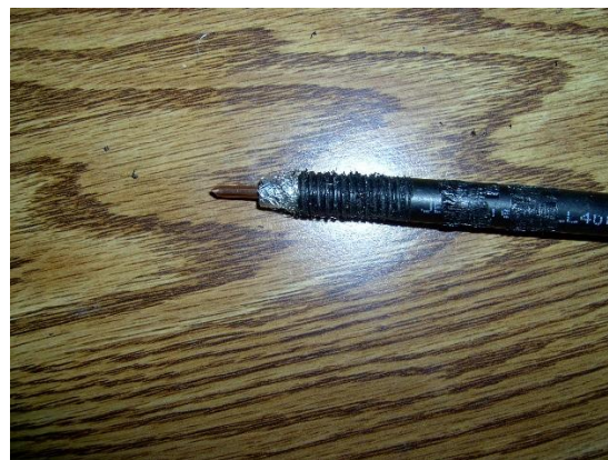
Approximately 1 1/2 inches of Threads Cut
