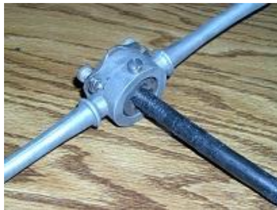
Cutting the Threads into the Coax Jacket
