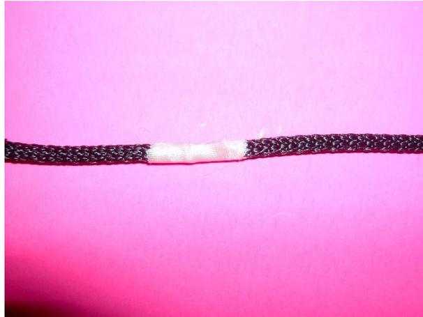
It is important that after cutting the rope that the ends are sealed properly. If not, the outer braid jacket will creep back up the rope exposing the inner braided core. This can cause problems.
