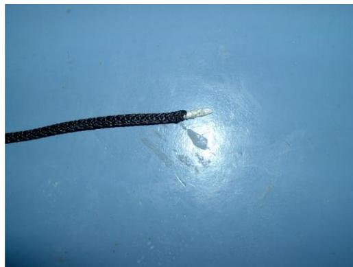
Using a flame, touch the taped end of the rope to the TOP TIP of the flame long enough to create a molten bead of rope material. Remove the flame and pull the molten end with a cloth rag (Don't use a paper towel- this stuff is HOT and will burn you). This will taper out the molten material so there is a concentric molten seal as well as not leaving a "bulge" at the rope end. (A bulge would increase the rope diameter at that point possibly causing pulley interference or knot tying problems).
