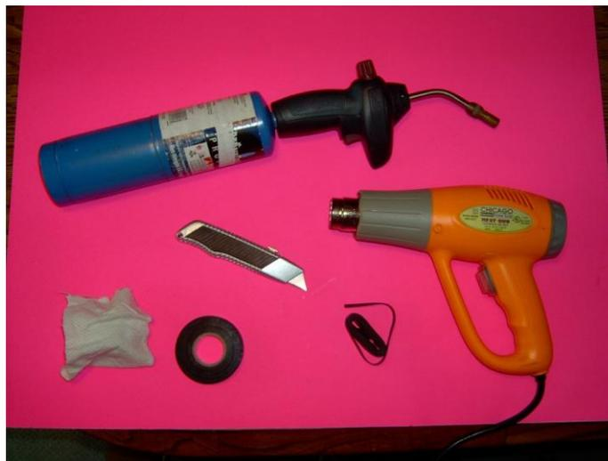
Propane Torch, Heat Gun, Utility Knife, Rag, Vinyl Electrical Tape, Heat Shrink Tubing
